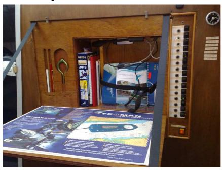
It has 12V power for an internal red light for chartwork at night, and the "library" was designed deep enough to take a Reeds Almanac. There are also USB connections for when I put the PC on the table, and the PC can then be connected to the GPS, and AIS (but not the Autohelm –yet!).
